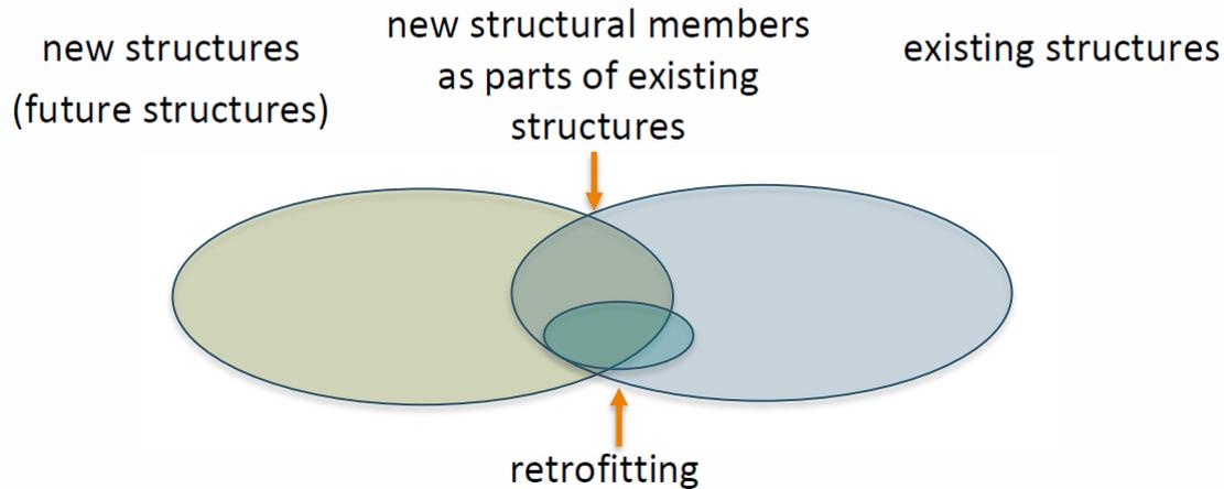
New structures and existing structures are not always easy to distinguish (overlap region is very important for engineer's activity)
